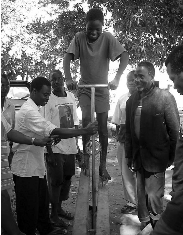
Figure 2: A treadle pump adapted for use by people with reduced strength
